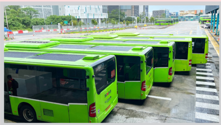
Solar panels are fitted on the roof of diesel buses
