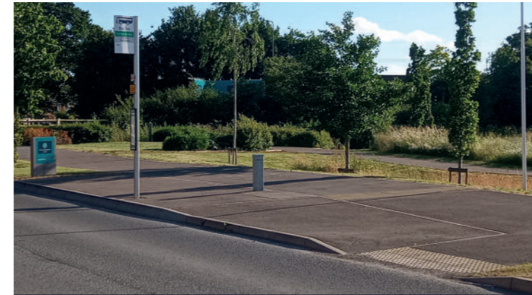
Fig. 38 Minimum bus stop infrastructure should incorporate a level paved boarder of sufficient size to accommodate a wheelchair ramp, a dropped kerb, a quality flag and timetable case. This flag has been incorrectly installed with the case facing the carriageway: a mistake as common as it is foolish.
