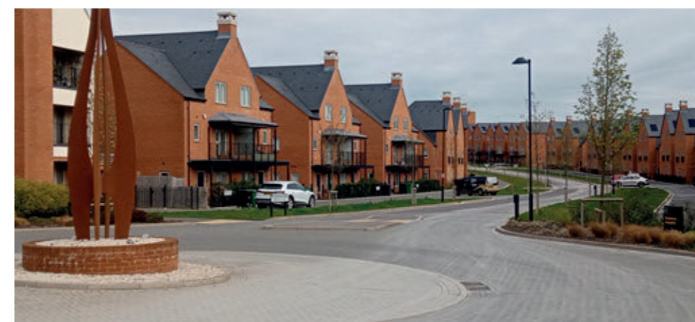
Fig. 15 The generous scale of the primary boulevard accommodates planting, swales and two parallel shared space serviceways which act as quietways for cycling. While relatively unusual, this is entirely consistent with the National Model Design Code.
