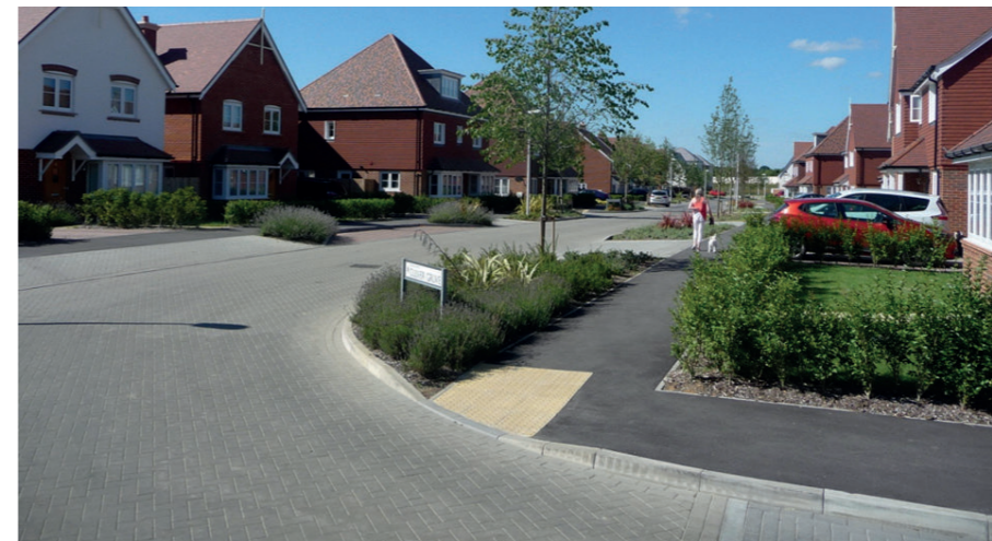
Fig. 46 Wokingham Northern Urban Extension - This street achieves an excellent balance between multiple urban design requirements. Parking in front of plots, and lavish planting, can co-exist while keeping a carriageway largely free of parking.
