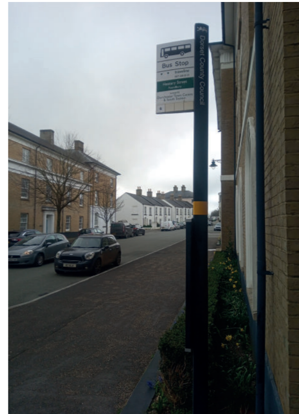
Fig. 27 Bus stops should never impinge directly on habitable windows. Even more care is needed where shelters are concerned adjacent to built frontage.
