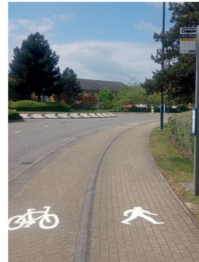
Fig. 36 Physical protection of bus users from passing cycles and micro-mobility cannot legitimately be compromised. Where width does not permit fully compliant segregation, including boarders, then cyclists should be expected either to use the carriageway, or off-line high-quality segregated provision on a parallel route.
