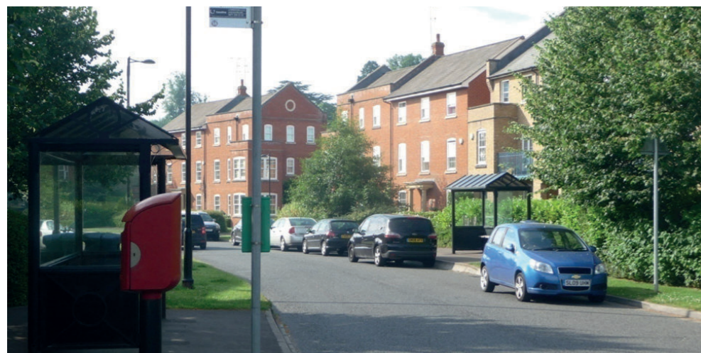
Fig. 30 Illegal and inconsiderate parking makes it impossible for bus stops to be used safely. Parking bays or a stop buildout would have been appropriate in this street.
