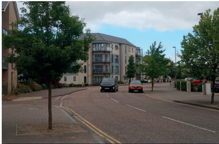
Fig. 4 Appropriate road curvature reduces speed without an excessively tortuous alignment.
